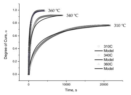
Figure 1: Comparisons between the calculated and measured degree of cure versus time.
